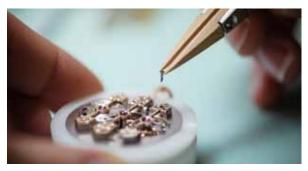
Assembly of the three gold Bridges on the movement
